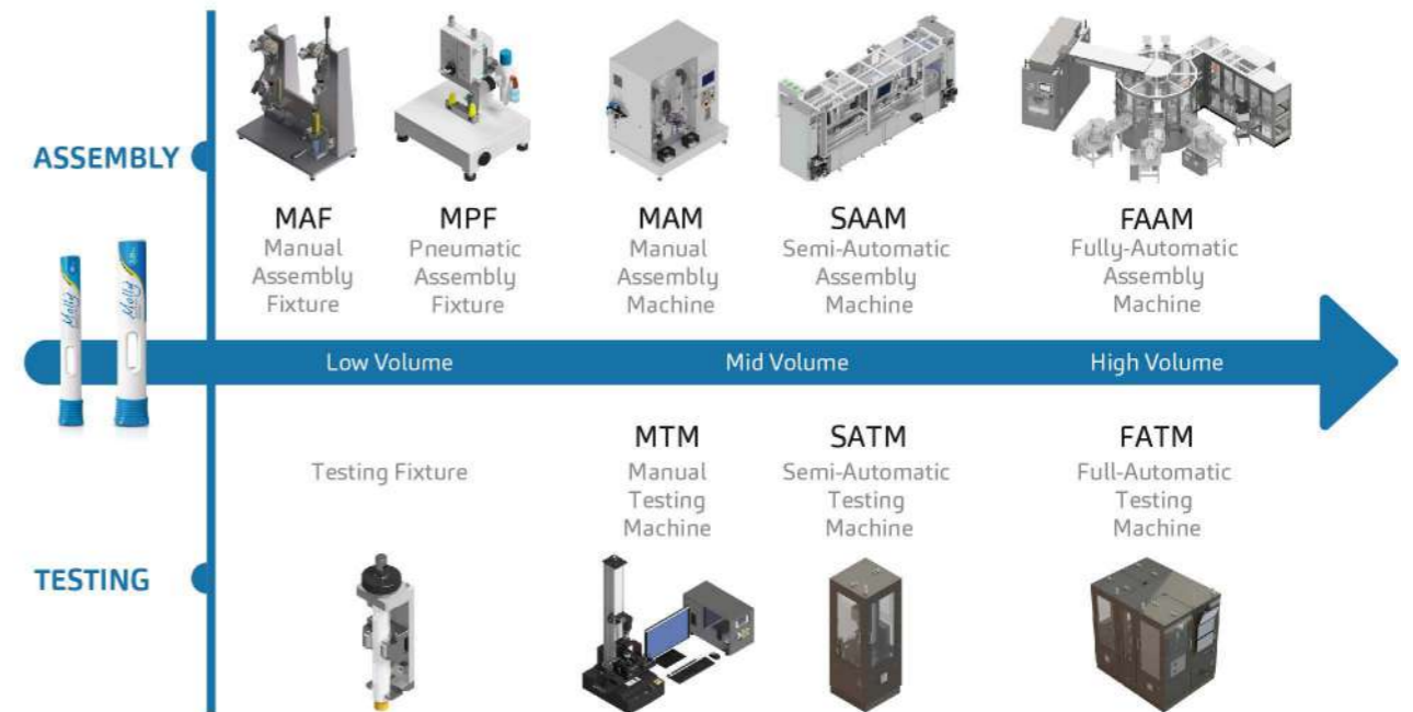
Figure 11: An overview of SHL Medical's modular assembly and testing machines that support varying requirements of Molly device projects.
